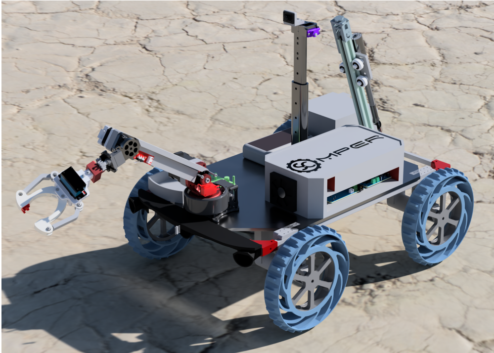
Figure 1: Conceptual design of the MPER system. The active chassis is designed to stabilize the central platform for the manipulator and drill.
