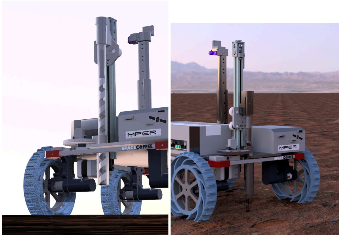
Figure 6. Renders of the drilling system in the stowed (left) and deployed position (right). Note the guide, one part of it extending with the motor (attached to the gantry). This allows travel of the drilled sample upwards.
