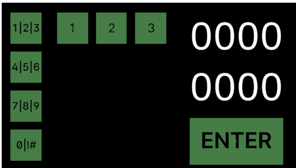
Figure 5. Third Design of a BCI numerical keyboard, with the first menu open
