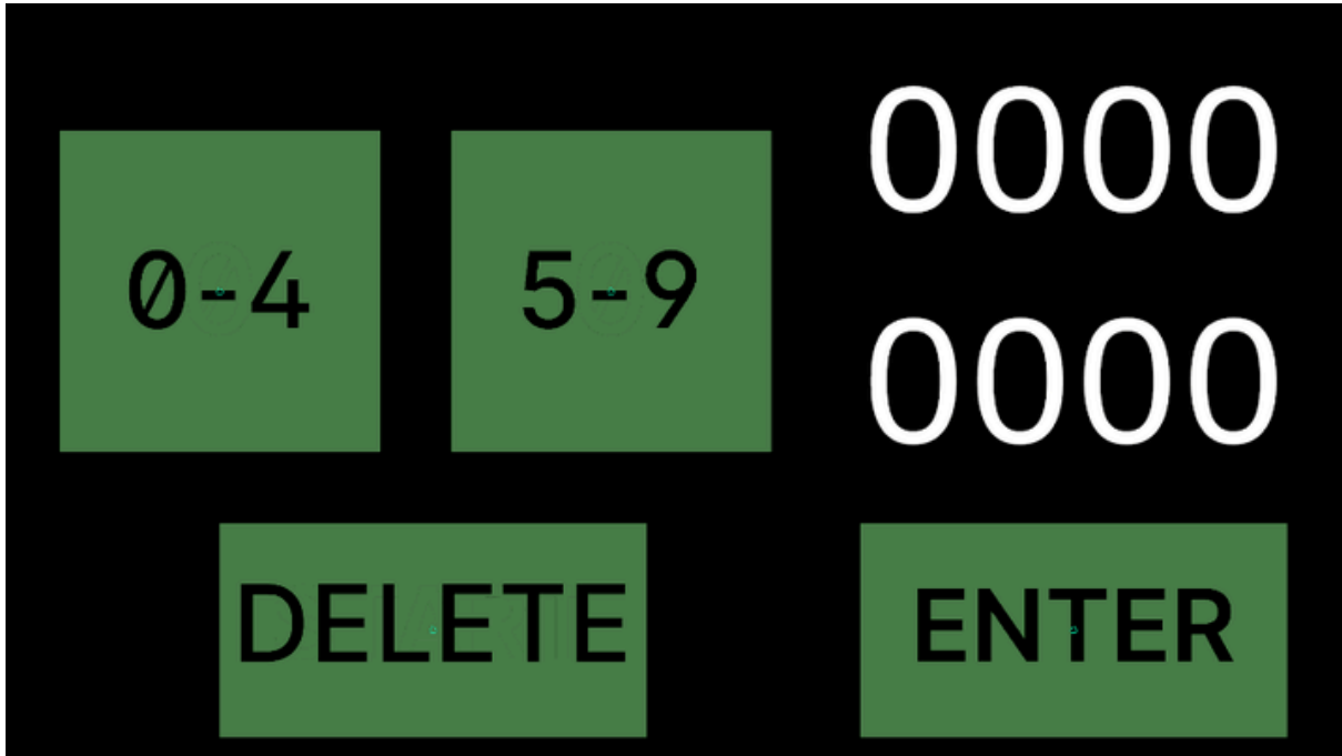
Figure 7. Fourth Design of a BCI numerical keyboard, with the main menu open
